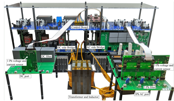
Fig. 7: Transformer hardware prototype with SiC BiDFET-enabled three-phase AC/DC converter
